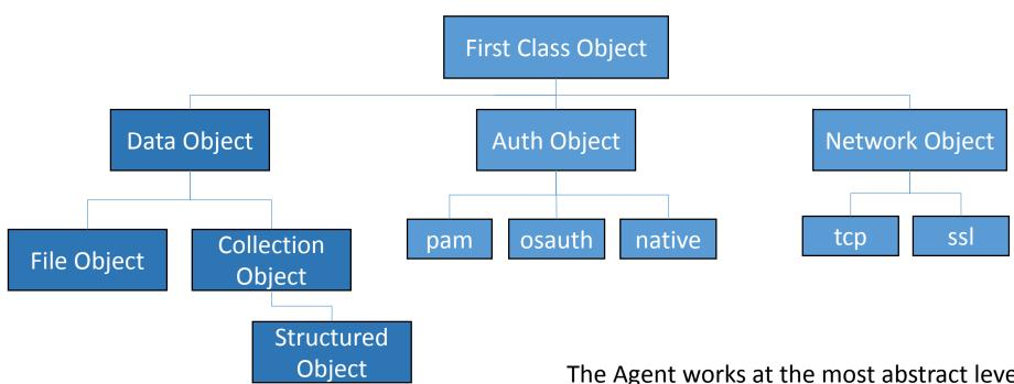
The Agent works at the most abstract levels in their hierarchies: the *plugin\_base* class and *first\_class\_object* levels. If a *first\_class\_object* resolves a plugin, the system assumes the plugin can operate on that first class object.
