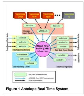
use this facility to extract metadata automatically from a data stream. The Antelope System uses a relation-based database called Datascope which stores metadata in a relational schema as well as storing sensor data. It exposes a relational view of accessing sensor data as rows and allows time-interval querying. The ARTS system is used by multiple projects [26-29], including the SciON project [30], part of the DFC.
