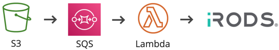
Figure 3. S3 to Simple Queue Service (SQS) to Lambda to iRODS
